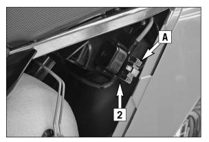
The fuse [1] is located in the starter relay of the E-starter [2] underneath the left side paneling.
